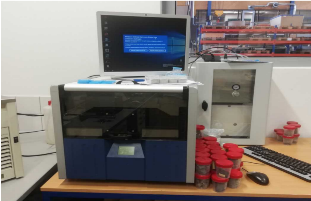
Figure 4.1: External view of the dynamic vapor sorption machine setup.
