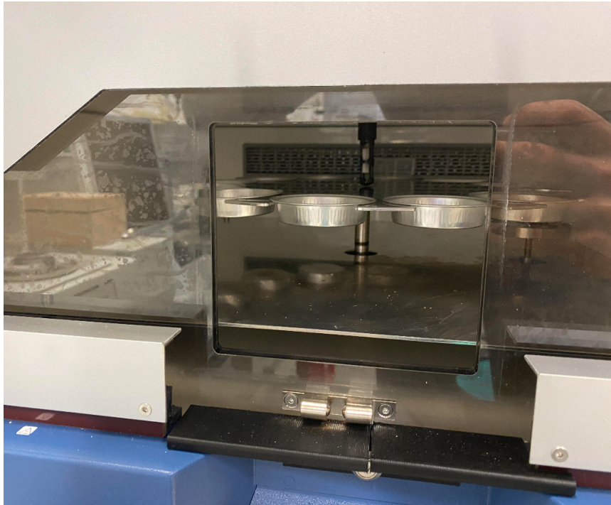
Figure 4.2: Internal view of the DVS machine chamber showing sample placement and humidity control components.
