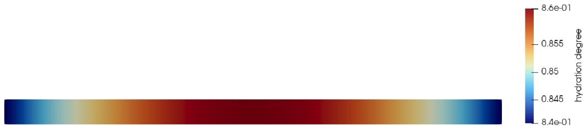
Figure 6.16: Spatial evolution of the hydration degree across the domain for a wall thickness of 40 cm at t = 3 d.
