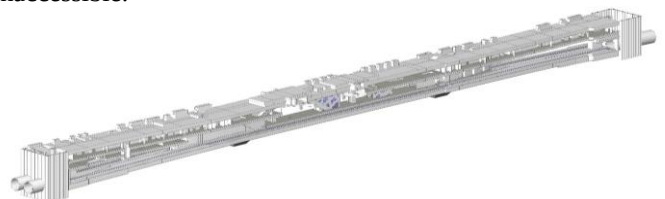
Figure 1. BIM model of a new subway station.
