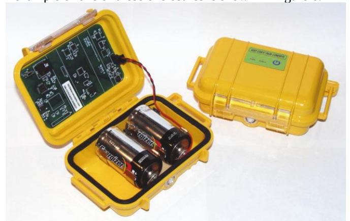
Figure 6. MEL accelerometer and enclosure
