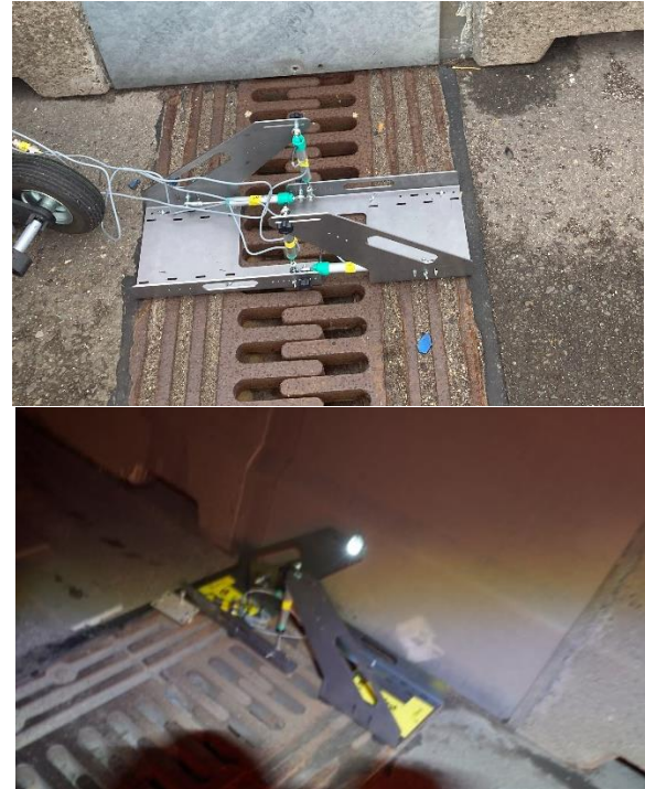
Figure 6. Midspan joint custom displacement sensor
