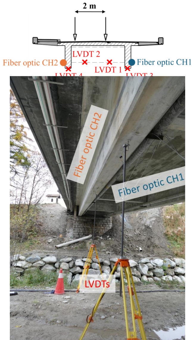
Figure 7. Sensor configuration. (Up) Cross section in one quarter-span for the load configuration LT3; (Down) Photo of the bridge with sensor locations.
