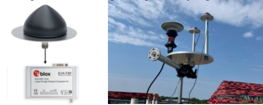
Figure 1: Left- Tallysman TWI antenna and U-blox F9P receiver, Right: The movement simulation device
