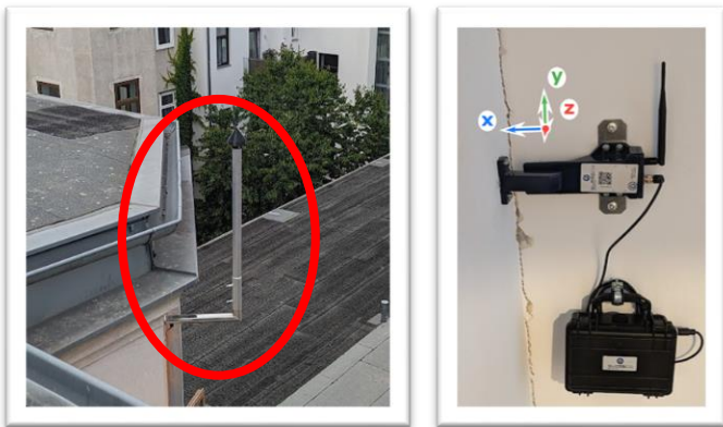
Figure 10. Left: Mounted GNSS antenna on the exterior wall of the residential building. Right: 6D sensor mounted in a building corner near the GNSS antenna.
