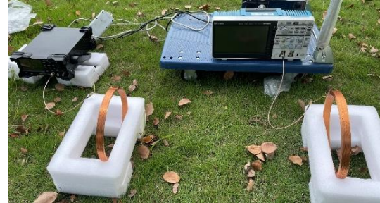
Figure 3 Outdoor Transmission Experiment Platform for Magnetic Induction Signal Using Mutual Inductance Coils
