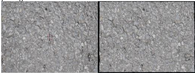
Figure 11. Synthetic asphalt pavement surface (left) and its 3D reconstruction with 10 \mu\text{m} spatial resolution (right).
