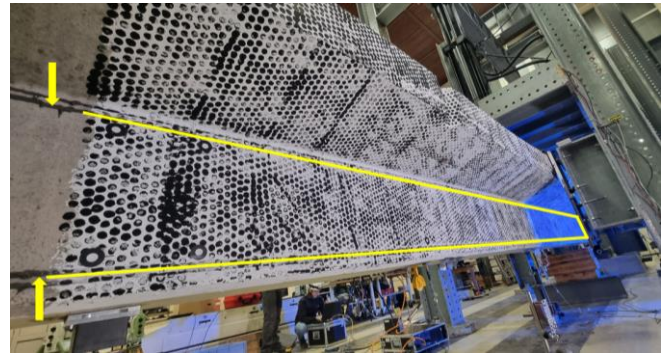
Figure 3. Glued fibers on the bridge girder placed in the laboratory.
