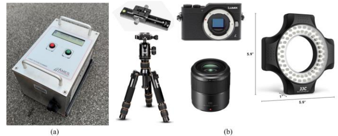
Figure 15. Apparatus of field texture scans: (a) LTS model 9200, (b) 4K camera, macro lens, tripod, slider, and ring light.
