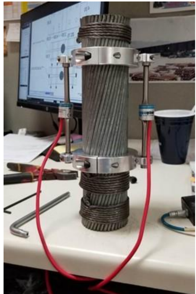
Figure 3. Prototype strain gauge assembly.
