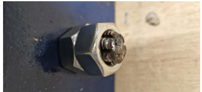
Figure 13. External thread used for the application of a threaded nut on an anchor strand.
