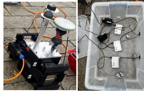
Figure 6: Left- The APS 113 shaker used for the experiment with Tallysman TWI, U-blox Patch and Leica AS10 Geodetic antennas. Right- U-blox F9P receivers connected to the antennas and Raspberry Pi devices to log the data.
