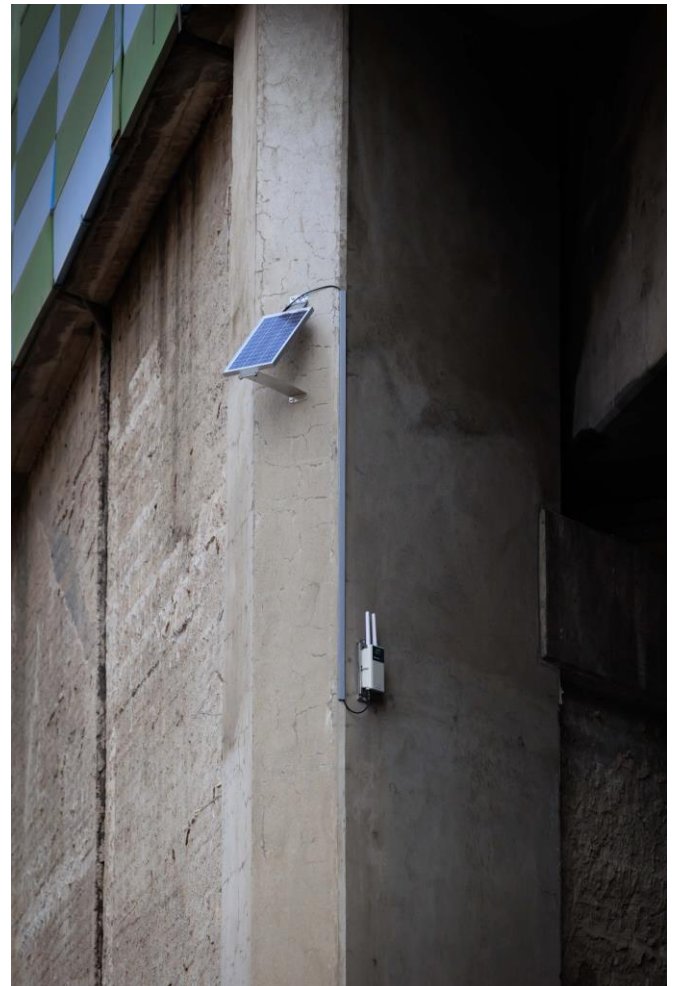
Figure 2: Wireless Sensor Nodes: 3-Axes-Tilt-Sensor (Triaxial Tilt Sensor) (Foreground) and Laser Distance Sensor (Background)
