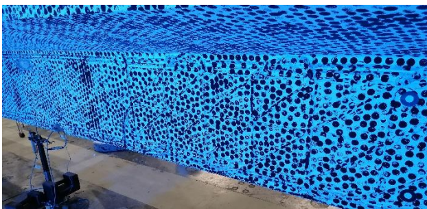
Figure 5. DFOS grid covered with DIC speckle pattern
