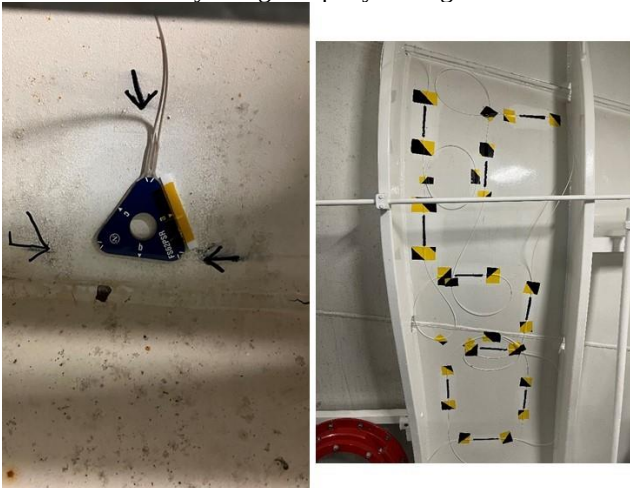
Figure 4. Rosette sensor on the Gadus (left) and chain sensor on the Jákup Sverri (right).
