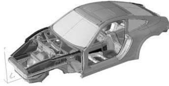
Abb. 4.41: Rohbaumodell eines PKW in SFE-CONCEPT [97]
