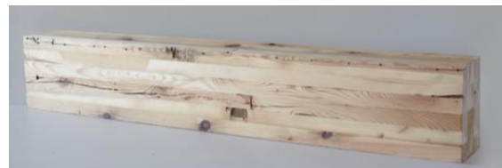
Figure 7. Glulam timber beam, with lamellas joined in vertical and horizontal direction
