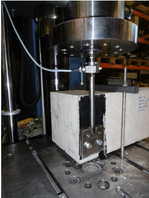
Figure 12. Experimental Setup of the peeling and pull-out tension test with Loop-Fastener. The width of the test strip is 5 cm. [10].
