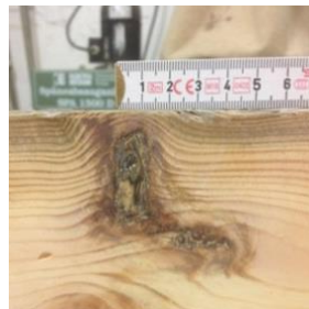
Figure 3. Strength grading: assessment of defects, decays, cracks and dimensions, location + orientation of branches
