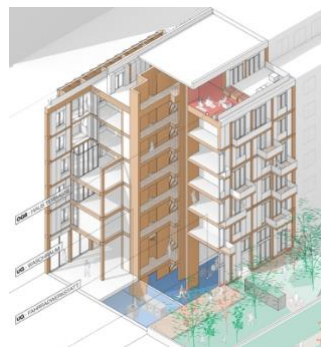
Figure 23. Skeleton system with stiffening core
