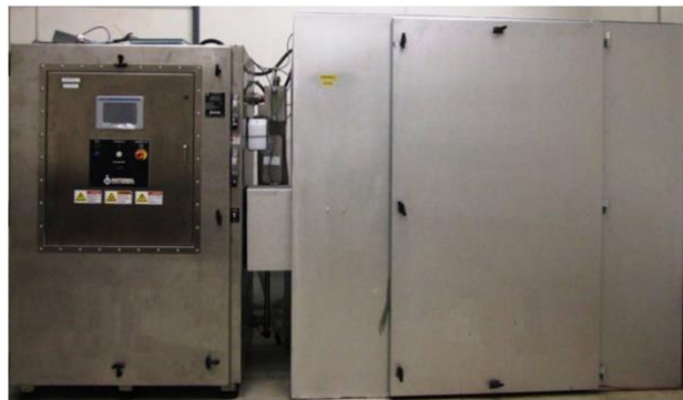
Figure 3. Pilot microwave heating system used for experimental program
