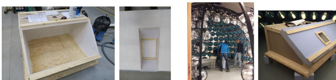
Figure 6. Measurement of daylight distribution. Model 1:4 (left) of a typical small room equipped with one roof window in the center, swappable roof for testing of various side linings. Preparation in the artificial sky-laboratory (right)
