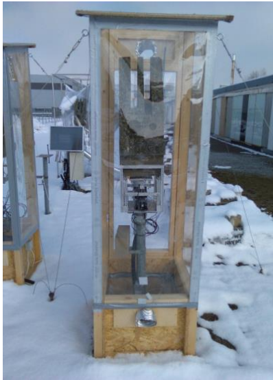
Figure 7. Newly developed foil enclosure in field test.
