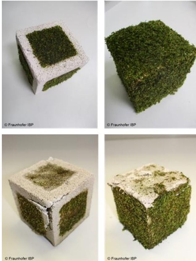
Figure 4. Three-dimensional test specimens of 10 by 10 by 10 cm AAC block and planted with moss (two different shapes). Test specimens before (top) and after winter weathering (bottom).
