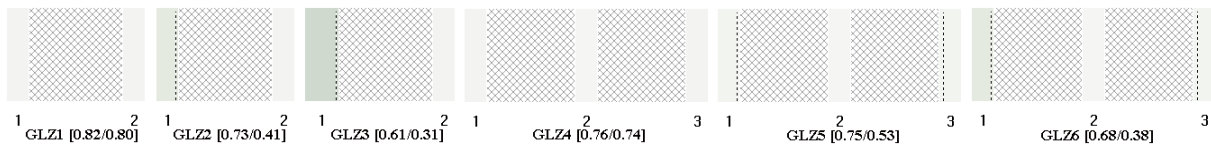
Figure 2. Coating position within glazing; 1- Outer glass pane Dotted line: position of coating(s)
