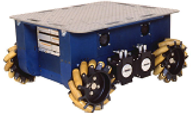
Fig. 5: Four Swedish Wheels - Uranus 5
