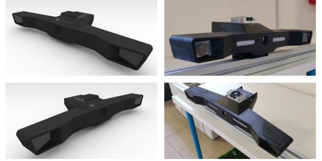
Fig. 1: The proposed sensor: renders (left column) and its realization with a really functioning prototype (right column).
