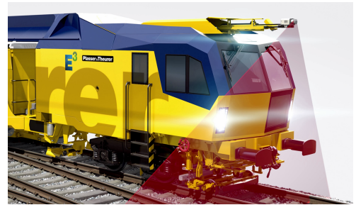
Fig. 1. Tamping machine with a roof-mounted 3D laser scanner.
