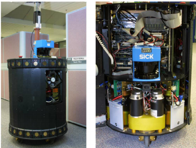
Fig. 4: Four Castor Wheels with eight motors - Nomad 4
