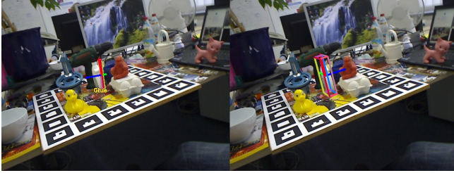
Fig. 4. Warped 3D box detection of the object glue
