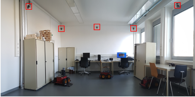
Fig. 7: Case studies laboratory, IR-cameras indicated in red.
