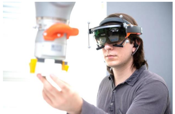
Figure 1: Human-robot collaboration and intuitive interface (HoloLens, eye tracking, markers for OptiTrack localization) for the assessment of human factors state to characterize key features in the collaboration domain.
