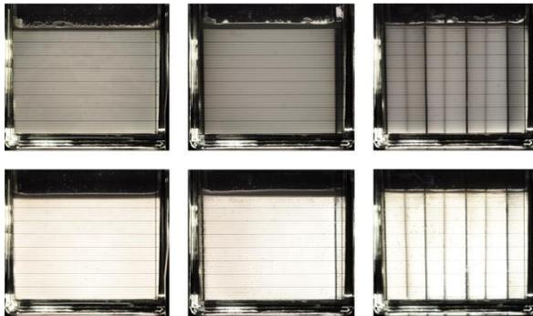
Fig. 3: Optical comparison of dispersed phase separation. Gravitational field (left hand side), plate-plate geometry at 120 V/m (middle) and plate-rod geometry at 200 V/m (right hand side); the upper pictures show the emulsion at the beginning of each experiment the lower figures show the result after 180 min
