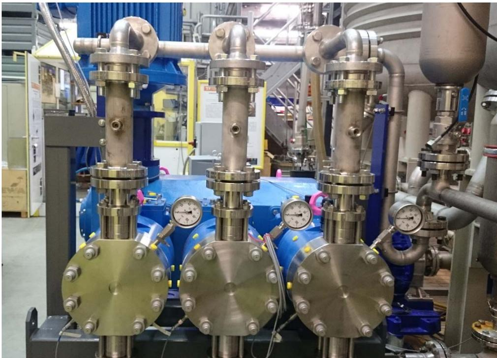
Fig. 2: The triplex diaphragm pump with three inline-pulsation-dampers
