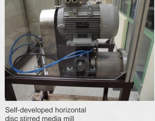
disc stirred media mill Volume: 5 dm<sup>3</sup> Operation mode: continuous/batch and dry/wet
