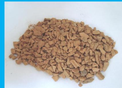
Figure 1. Crushed brick-fractions 0/4 and 4/8mm
