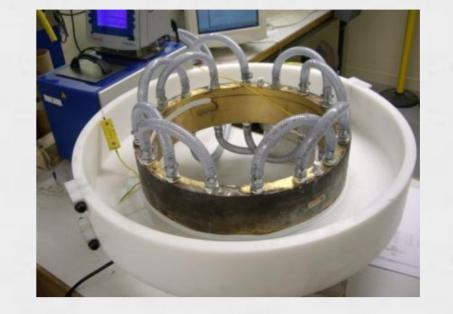
Ring test before casting
