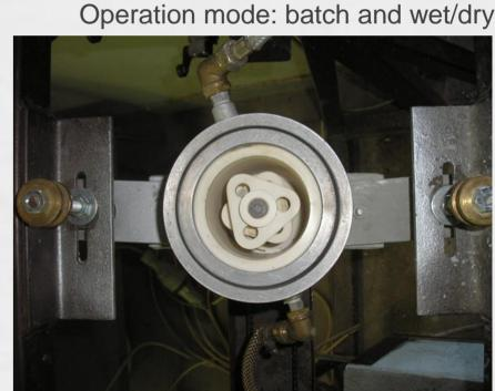
Self-developed horizontal disc stirred media mill Volume: 0.5 dm<sup>3</sup> Operation mode: batch and wet/dry
