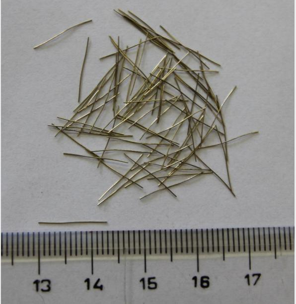
Fig.1 Micro-fibres used in the UHPFRC mixture (13×0.18 mm)
