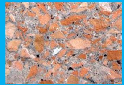
Figure 2. Concrete with 100% of recycled bricks aggregate and Concrete with combination of river and crushed bricks aggregate Table 2 Experimental results
