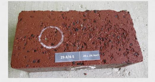
Fig 4. Surface of 2 paving stones after 28 cycles of freezing-thawing
