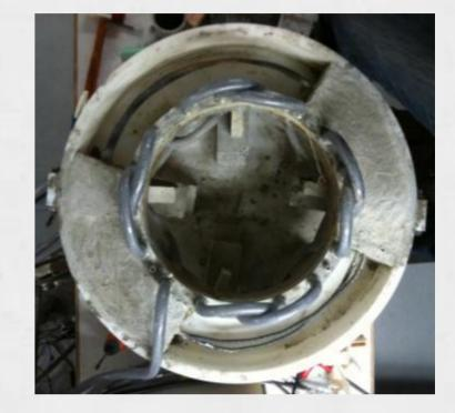
Ring test with rebars and construction joints
