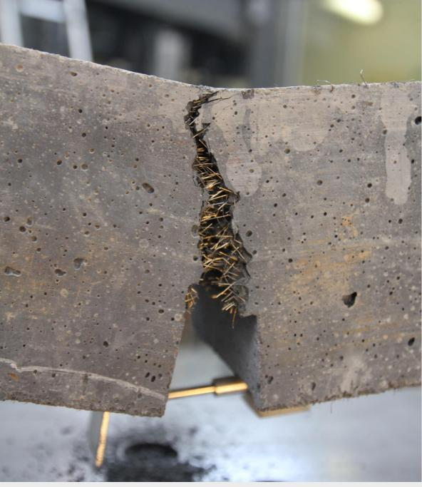
Fig.3 Fracture energy of the UHPFRC measured on the notched specimen
