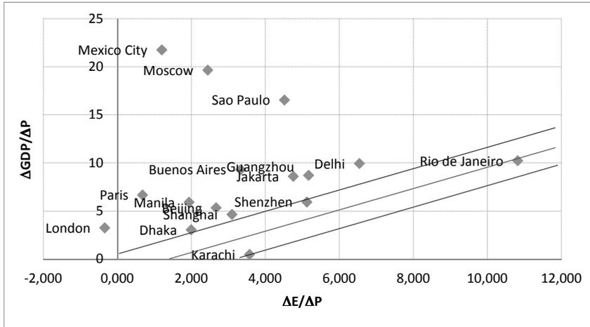
Figure 4 Name needed. Plot of growth ratios for GDP and Electricity consumption.
