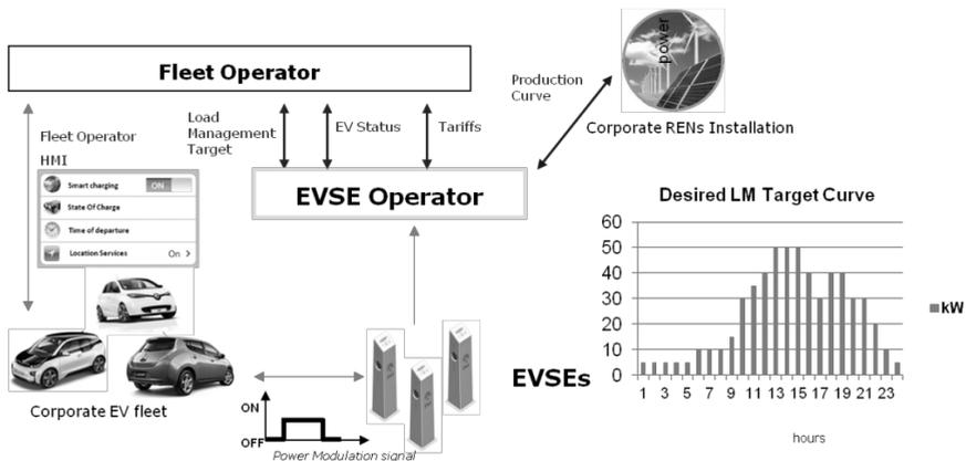
Fig. 5. Architecture of Electric Mobility Management system developed by Enel Group
