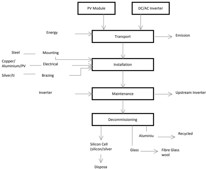
Figure 2: Flow diagram of rooftop PV System
